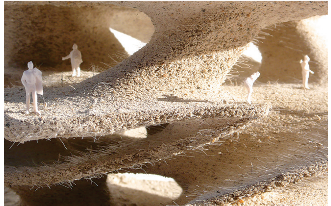
Detail of Earthscrapers , showing nylon fibers in sand print
