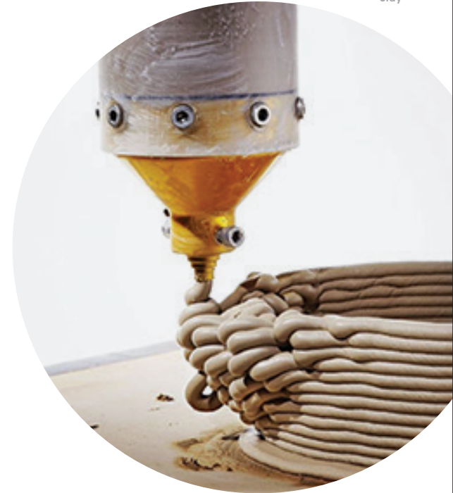
Potterbot paste extruder 3D printing clay
