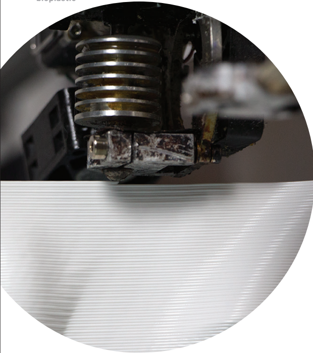
Fused deposition modeler 3D printing bioplastic
